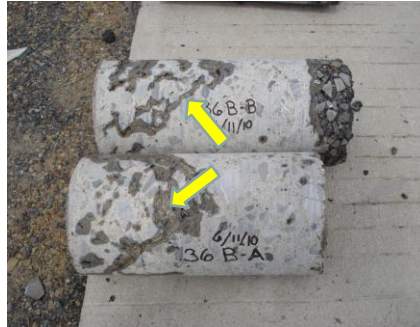
Cores taken from the pavement showing cracking below the surface
